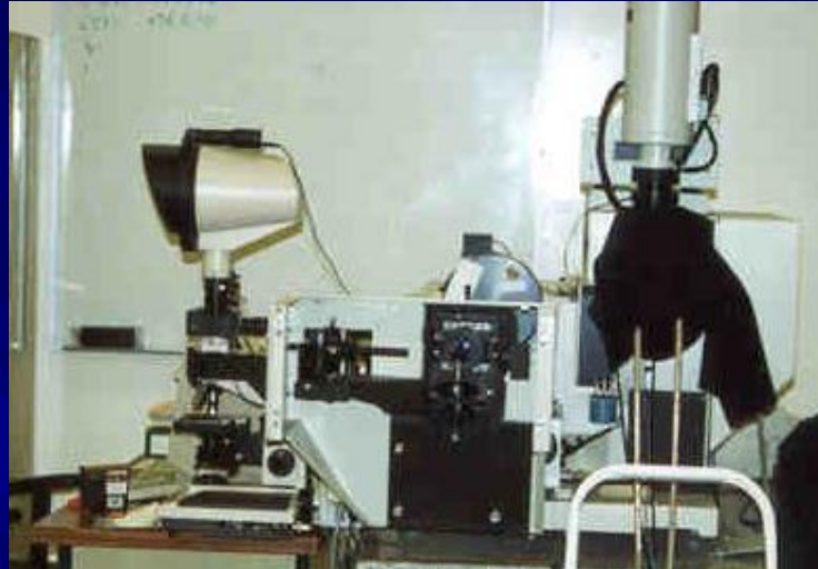
Micro-Raman system: 2D mapping of characteristic vibration modes of layers and coatings, e.g, graphene
