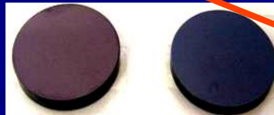
Hard colored nanomaterials produced by sputtering
