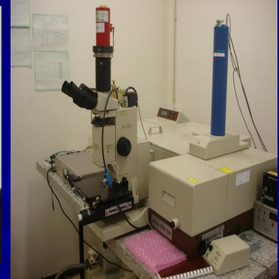
IR FTIR Spectrometer: IR transmission and reflection measurements in the spectral and temperature ranges of 10000-20\text{ cm}^{-1} and 20\text{K} to 500\text{K} , respectively.
