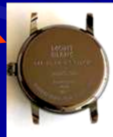
Hard colored nanomaterials produced by sputtering
