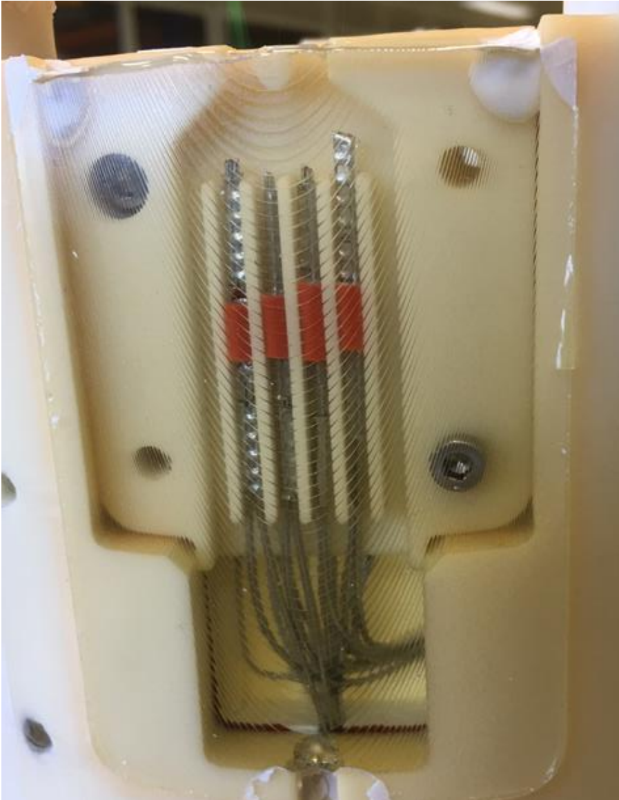
Impregnation test, the box will be filled with a glass filler, beads or chopped fibres for the final magnets
