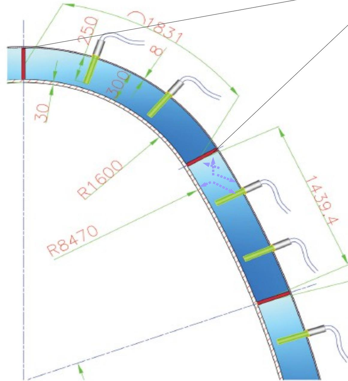
Construct a large detector segment of  $O(2\text{m} \times 2\text{m})$  with curved walls as close to vessel design as possible
