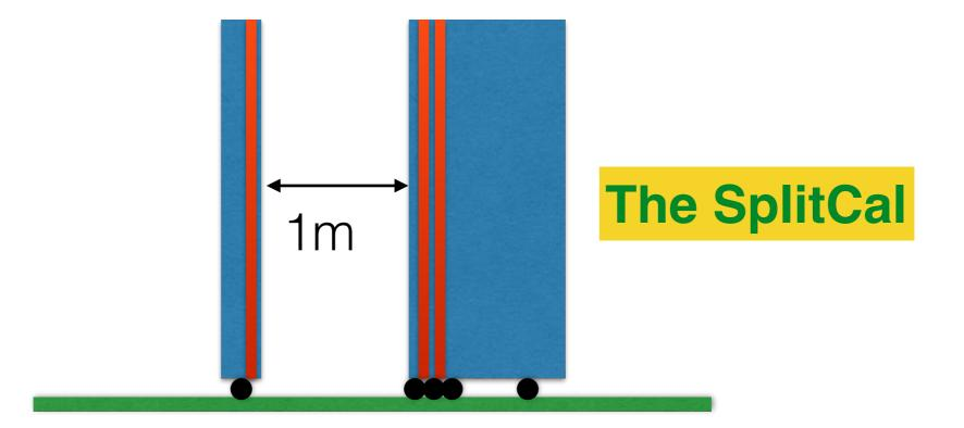
Implemented in FairShip and "tested" (with some cheating...) in blue a sampling Pb ECAL with X-Y plastic scintillator bars readout via WLS fibres from the sides (see our ICL June2016 talk)
