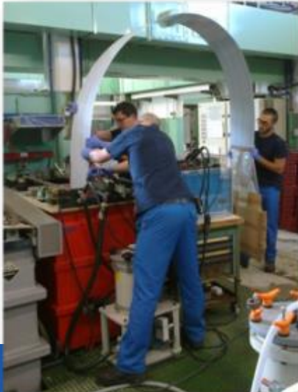
Ag plating on Al stripline contact AD
