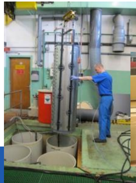
Cu plating on DTL tank of Linac 4
