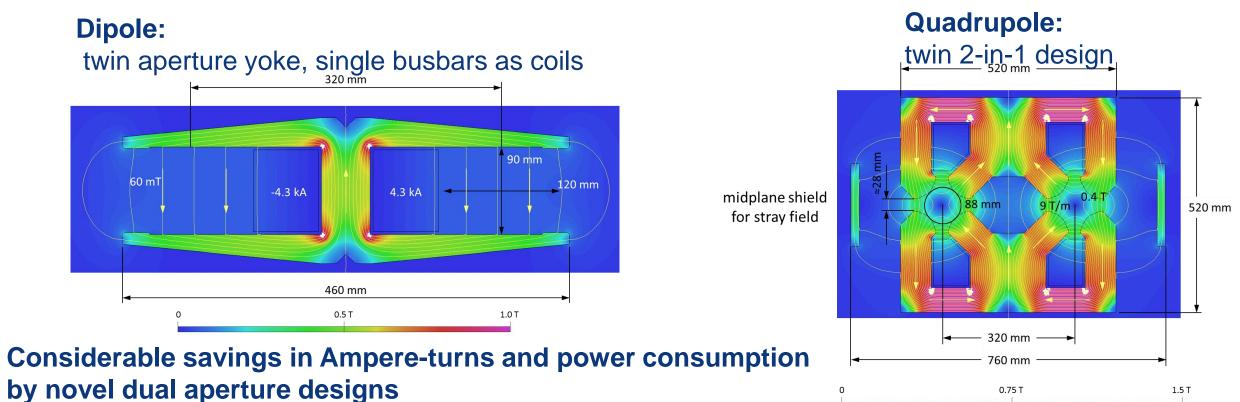
Power consumption twin quad: 22 MW at 175 GeV with Cu coil (half of single-aperture quads) and power consumption twin dipole: = 17 MW at 175 GeV with AI bus bar
