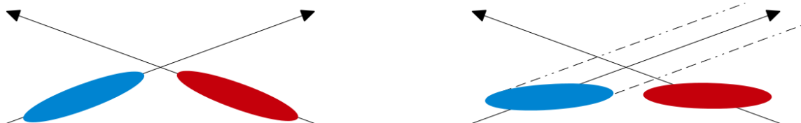
Figure 2 Schematic of bunches colliding with a crossing angle at the interaction point. Without crabbing (left) and with crabbing (right).
