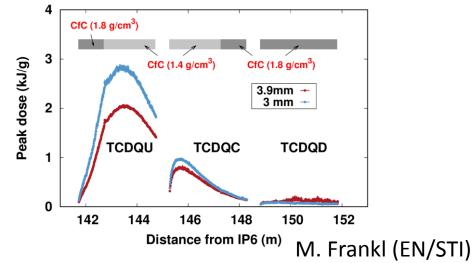
Constraints due to energy deposition in TCDQ (asynchronous beam dump)
