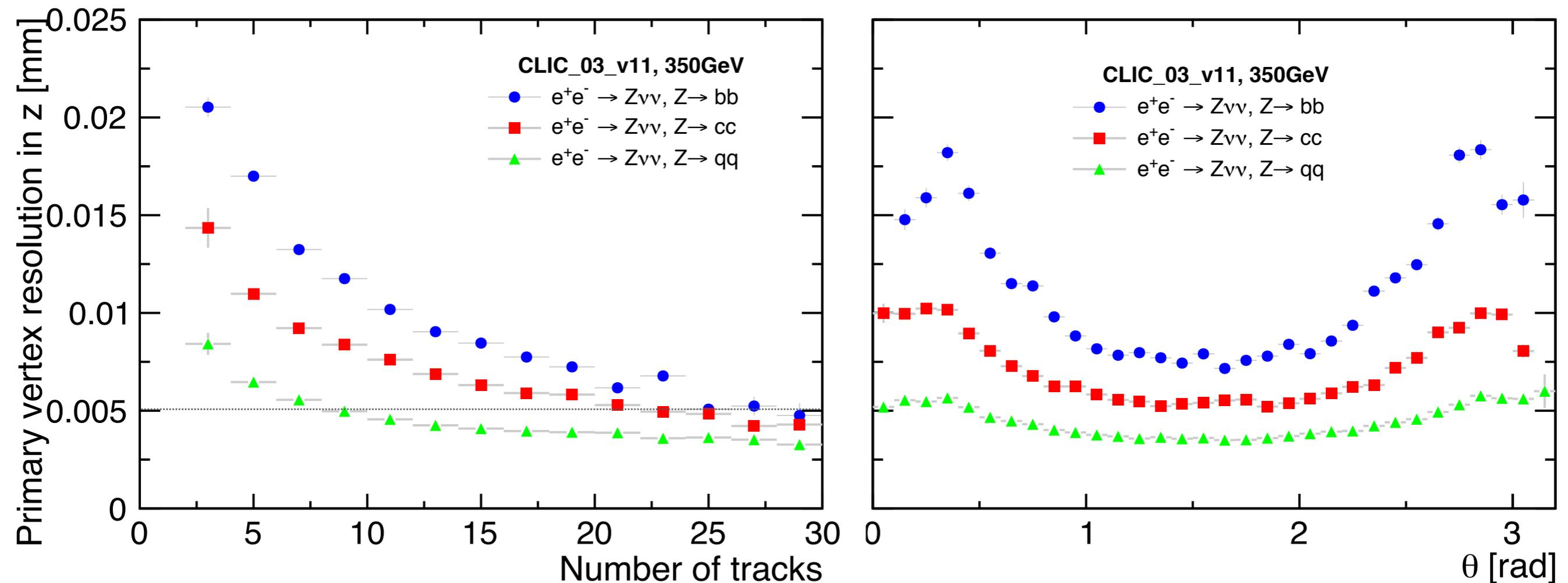
**Resolution of the PV versus the number of tracks and the angle theta**
