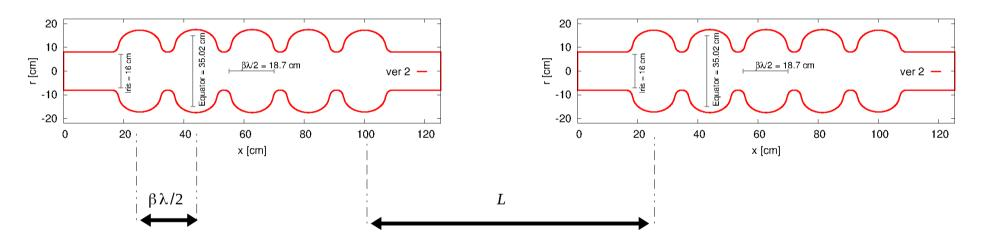
However, round trip time is ~30  $\mu$ s, so change in RF phase between passes is not feasible ( $\tau_{cav} \sim 8ms$ ). Is it possible with return arc tuning + fast cavity tuning<sup>1</sup> using piezo's/ferro-electric materials
