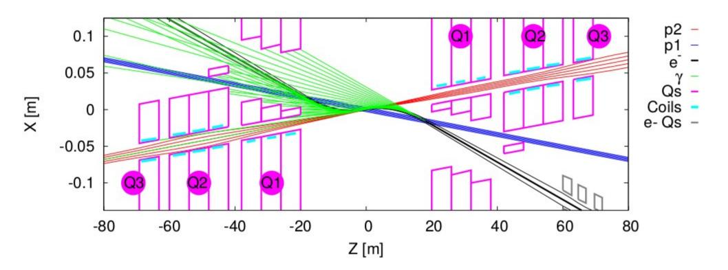
Scaling LHeC design leads to beta\*=20cm, L\*=20m, IR total length 1080m. (Goal is: beta\*=15cm in 700m)
