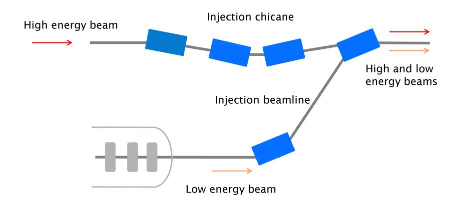
Beam injection studies required to ensure sufficient emittance preservation
