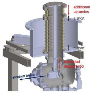
Maximum Voltage 548 kV Operational Voltage 450 kV Operational current 1 mA with GaAs
