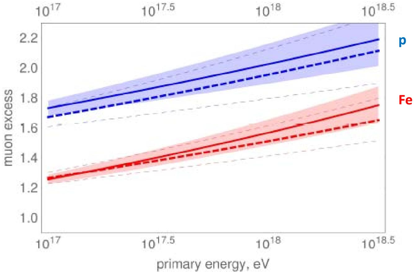
**The empirically determined number of muons with energies above 0.75 GeV exceeds the simulated one.**
