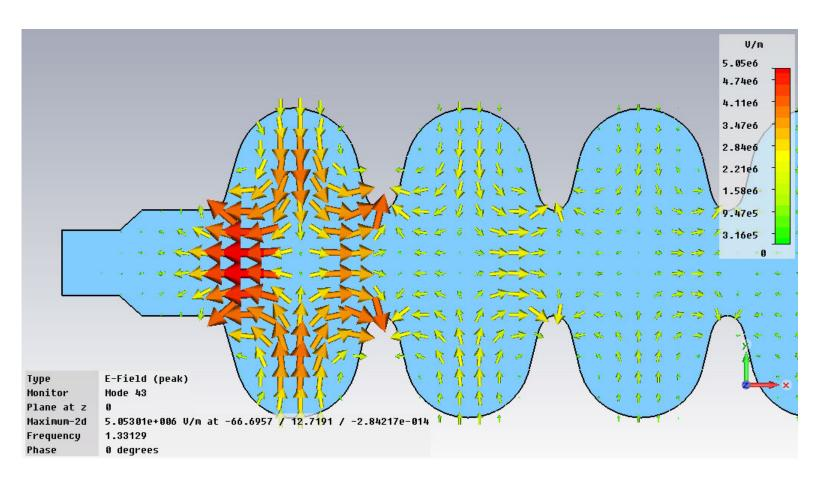
Evanescent fields since far below TM01-cut off in 40mm-beam pipe radius (~2.80 GHz)
