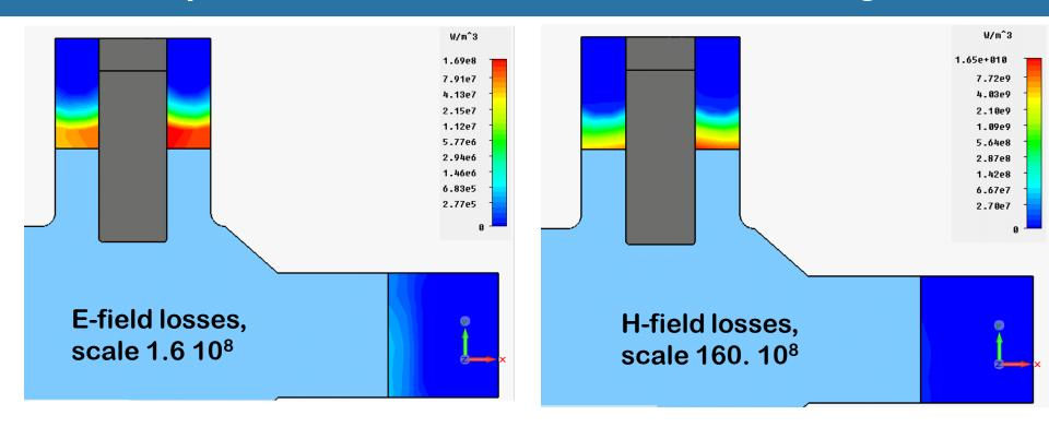
Computed Q<sub>ext</sub>: 16500; losses almost completely in the input coupler
