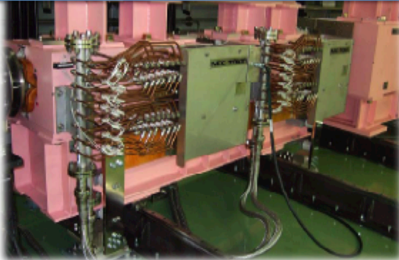
High field magnetic septa (SMS31,32)
