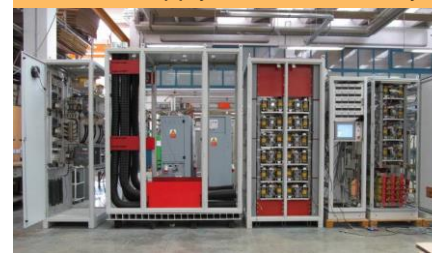
1.8 MW supply unit for MA cavity
