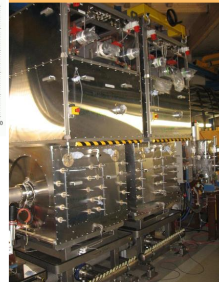
New MA cavities in tunnel
