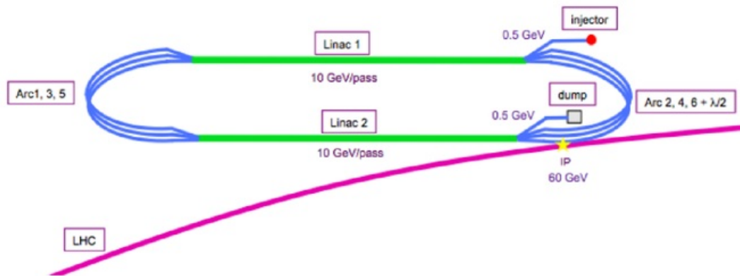
Figure 4: Diagram showing the proposed Linac Ring structure of the LHeC, with two 10 GeV energy recovery linacs arranged parallel to one another and tangential to the LHC [13].
