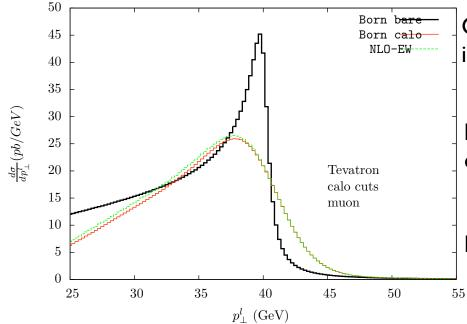
Calorimetric energy deposit is not pointlike but approximated. by gaussian distribution → smearing of the lepton momenta
