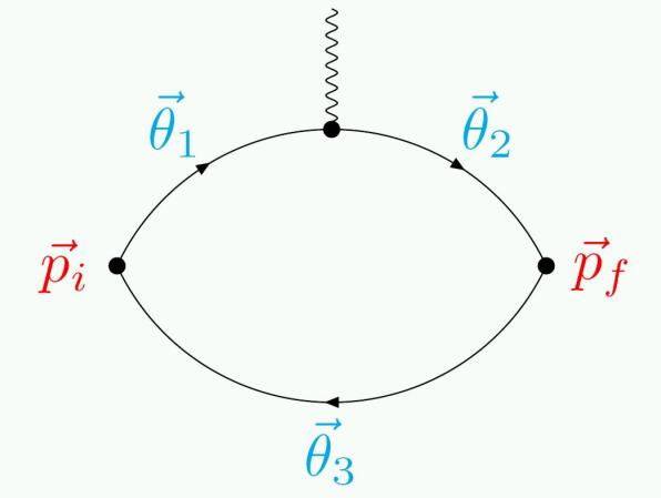
$$\begin{aligned}\vec{\theta}_i &= \vec{\theta}_1 - \vec{\theta}_3, \\ \vec{\theta}_f &= \vec{\theta}_2 - \vec{\theta}_3\end{aligned}$$
