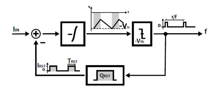
Cycle of operation (ideal) based on the charge-balance principle:
