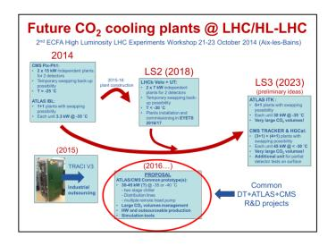
Roadmap for LS2 and LS3 CO<sub>2</sub> systems presented and agreed in the frame of the 2<sup>nd</sup> ECFA Workshop on High Luminosity LHC Experiments in October 2014.
