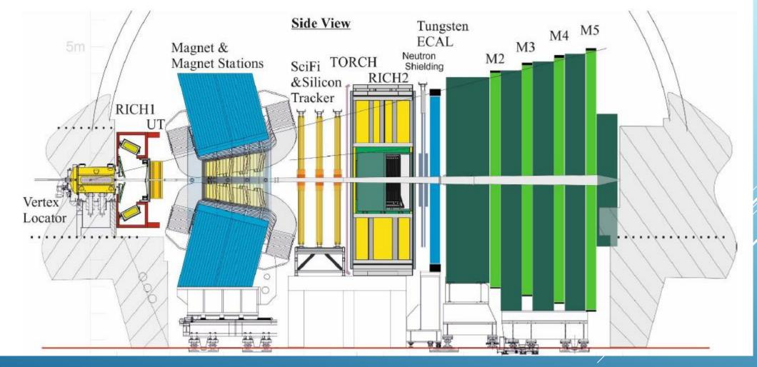
A massively upgraded detector is required. Smaller granularity. Precise time information appears like a must to disentangle overlapping events. VELO smaller pixels, precise timing, may replace after x years. RF foil thinned / removed?
