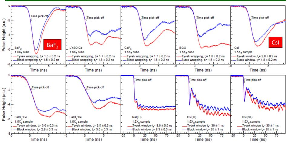
The 3 ns width of BaF<sub>2</sub> pulse may be reduced by a faster photodetector LYSO, LaBr<sub>3</sub> & CeBr<sub>3</sub> have tail, which would cause pile-up for GHz readout
