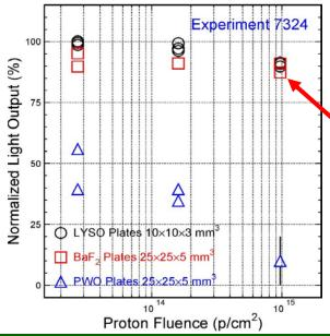
LYSO, BaF<sub>2</sub> and PWO plates of 3, 5 and 5 mm were also irradiated up to  $1\times10^{15}$  p/cm<sup>2</sup>.
