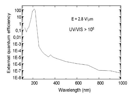
**Fig. 4.** External quantum efficiency extended to visible and near infrared wavelength regions. The
