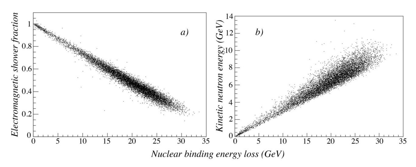
Results are for 100 GeV  $\pi$ - in lead absorber
