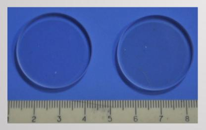
We got a few samples of a multilayer filters sprayed on the quartz glass substrate (KU-2 type) Quartz glass substrates are 30 mm in diameter and 3 mm thick
