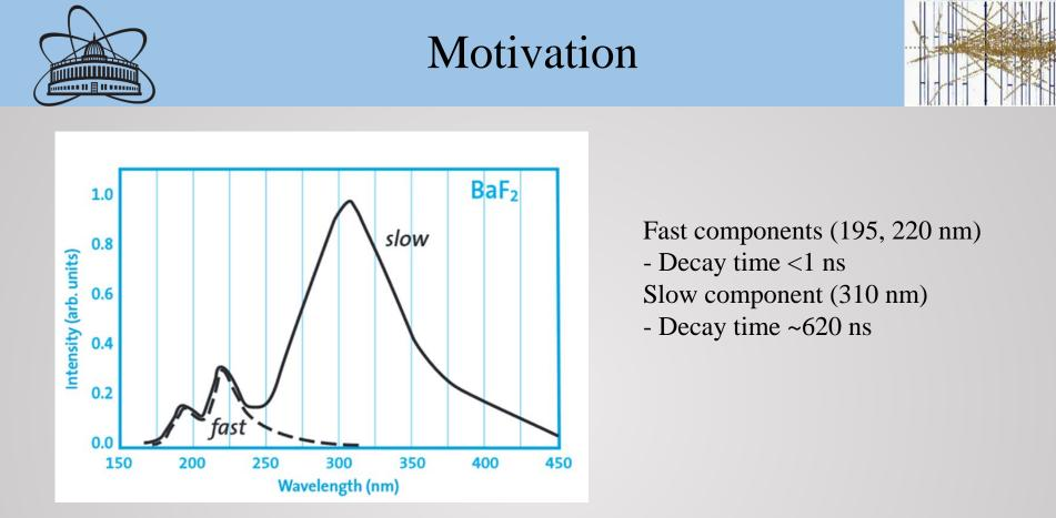
BaF<sub>2</sub> crystals are natural choice for the Mu2e-II calorimeter to use at the intensity frontier (see talk by Ren-Yuan Zhu).
