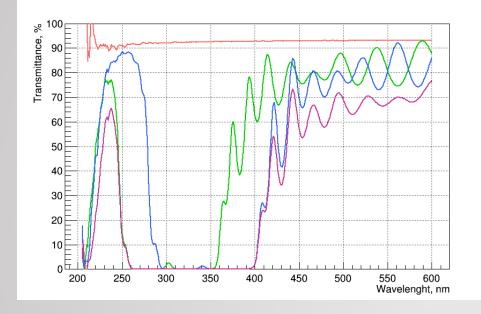
Transmittances of filters were measured with Shimadzu SolidSpec-3700 DUV photo spectrometer
