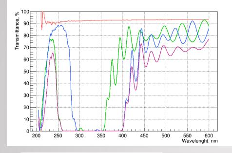
Transmittances of filters were measured with Shimadzu SolidSpec-3700 DUV photo spectrometer
