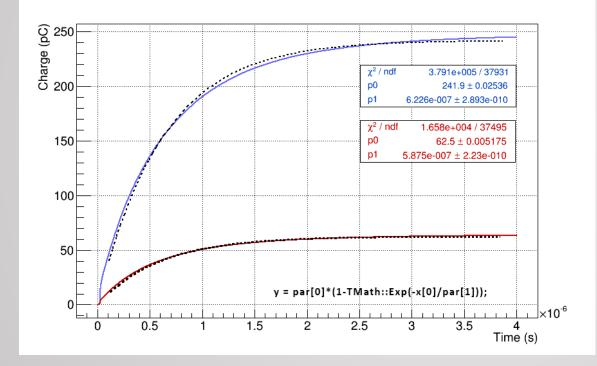
The averaged signal charges were calculated for the full range of digitization for a crystal with no and with a filter
