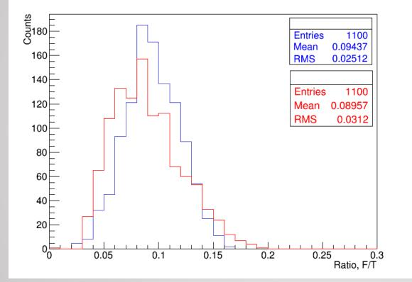
Fast/Total ratio was estimated by calculating charge due to fast component within 20 ns from the signal start and total signal within 2  $\mu$ s
