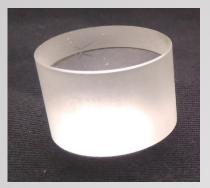
Crystal is 30 mm in diameter and 20 mm in height Two ends are polished, side is unpolished It was first attempt to spray a filter on the crystal: multilayer filter was sprayed on one BaF2 crystal end
