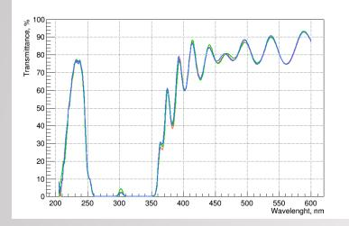
Three filters of "type 1" (top frame) as well as three filters of "type 2" (bottom left frame) were evaporated in different runs Three pairs of filters ("type1"+"type2") provide suppression of a slow component in the range 250-400 nm (bottom right frame)
