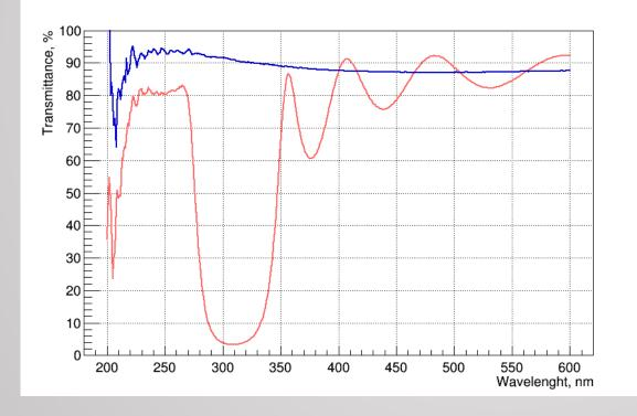
Transmittances: blue – dia. 38mm x 18 mm red - dia. 30mm x 20 mm
