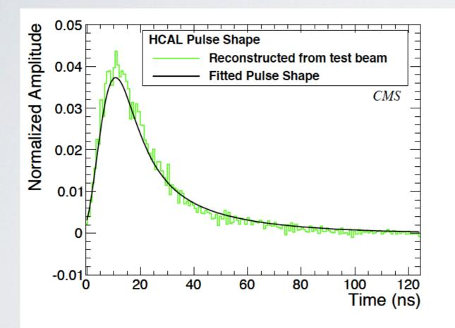
Figure 5: Average pulse shape reconstructed for the HCAL from H2 beam test data using 300 GeV pions.  New! QIEII time-to-digital converter (TDC) allows for in situ pulse measurements with Phase I readout
