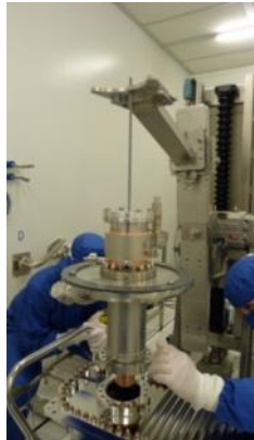
Assembly of the tube and window on the coupling box
