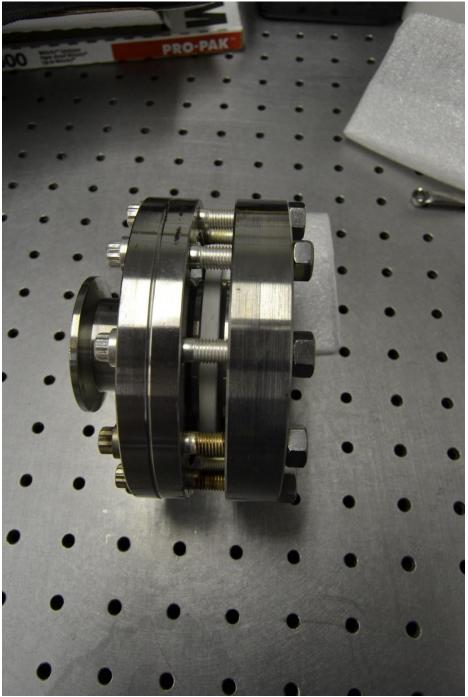
**Test 1:** (RT -> 0C -> RT -> 100C -> RT) x 10 times = OK (vacuum tight)
