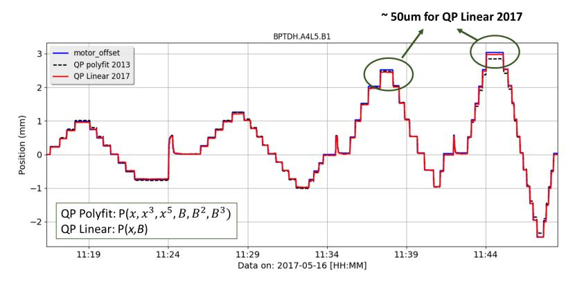
\*Jaw Gaps during scan: 14mm, 16mm, 18mm, 22mm
