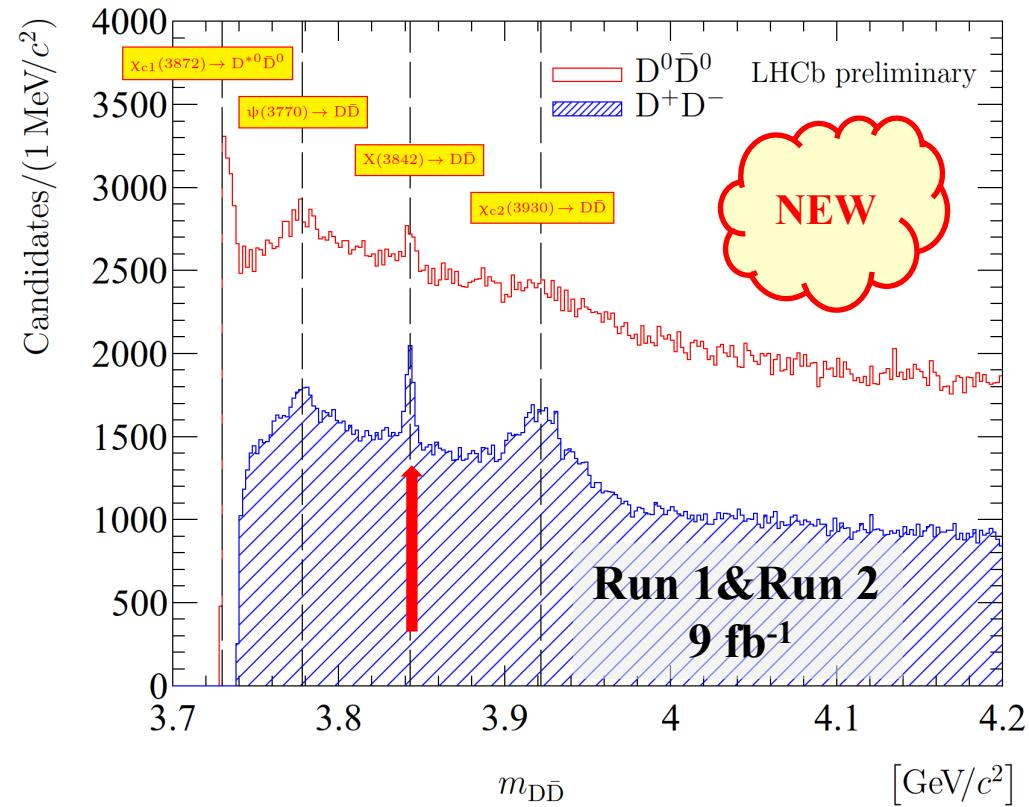
New narrow state **X(3842)** at open charm threshold is observed
