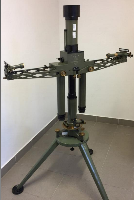
Eötvös-Pekár Balance ( Small Double Balance ) 1926, 1928, 1930
