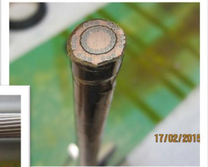
“2 kA coaxial cable”
