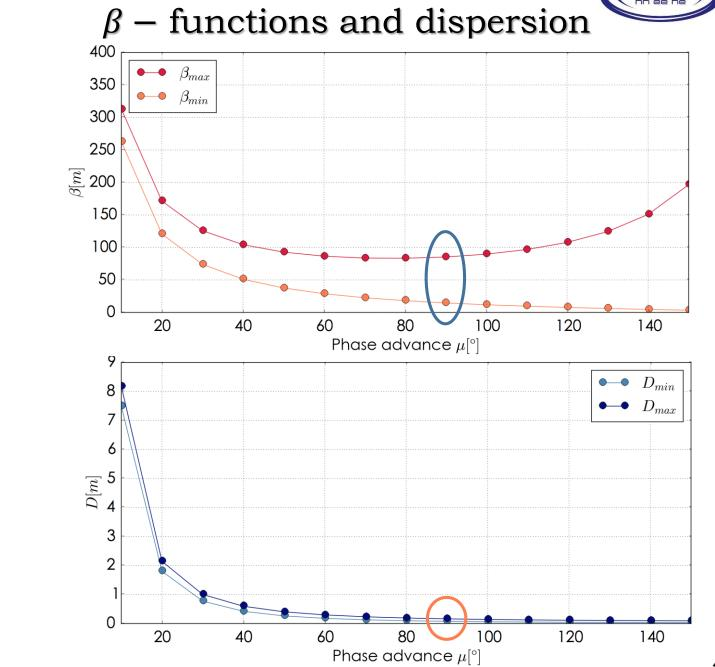
$$\beta_{max} = L_{FODO} \frac{\frac{1 + \sin \frac{\mu}{2}}{\sin \mu}}{\sin \mu} = 85.35 m$$
