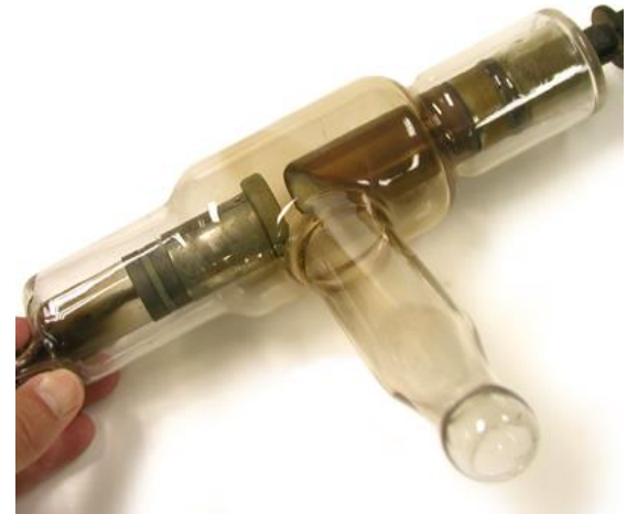
X-ray photo tube Credit: Oak Ridge Associated Universities, 1999
