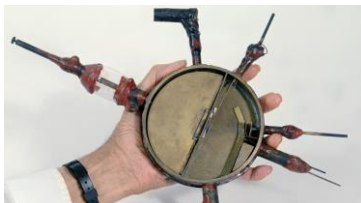
The first cyclotron, Lawrence Berkeley National Laboratory Photo Archives
