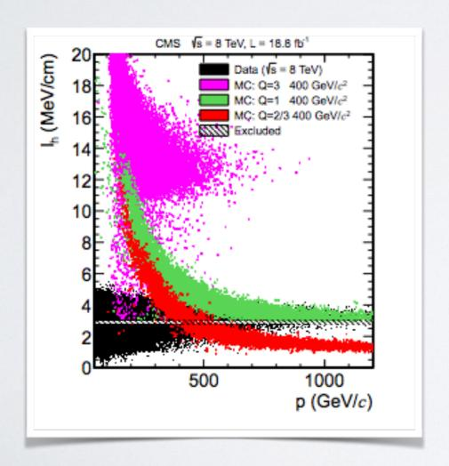
• dE/dx: Ionization energy lost. • TOF: Time of flight
