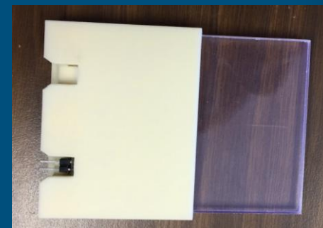
Scintillating tile 10 \times 10 \times 0.6 \text{ cm}^3 , each side equipped with 3 \times 3 \text{ mm}^2 SiPMs
