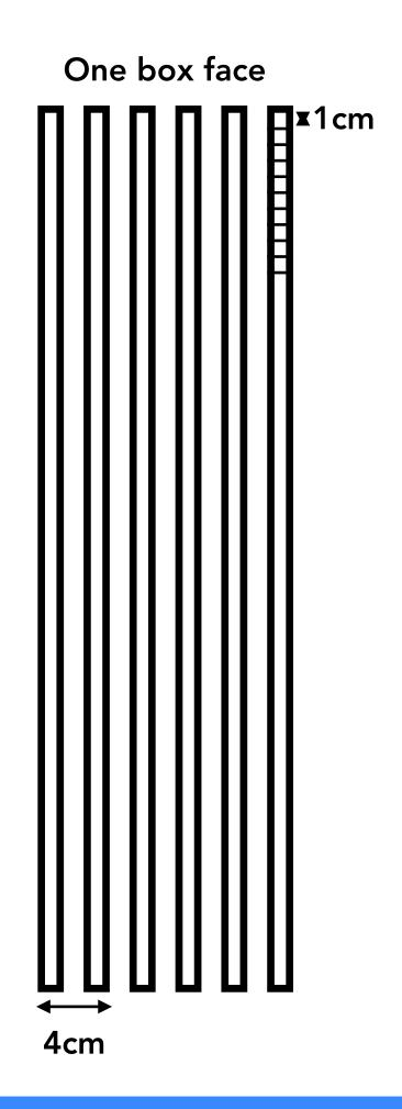
10x10x10 metre box, with 6 RPC layers on each box face. Assume 1 cm granularity for the RPCs, and possibility of timing information (explored later in talk). Add 5 other triplets of RPC layers equally spaced in box to minimize the distance to the first measured point for the decay vertex determination.
