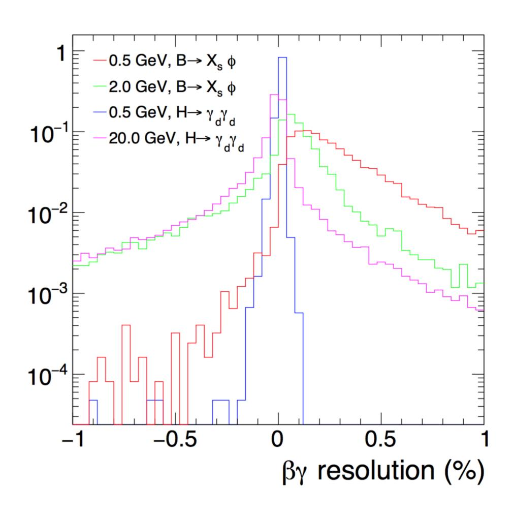
Reconstruct parent boost from the measured decay vertex (no timing!), assuming relativistic decay products. The resolution is < 1% (entirely dominated by distance to first measured point, not detector granularity) so the boost distribution is dominated by the generated spread of boosts, not resolution.
