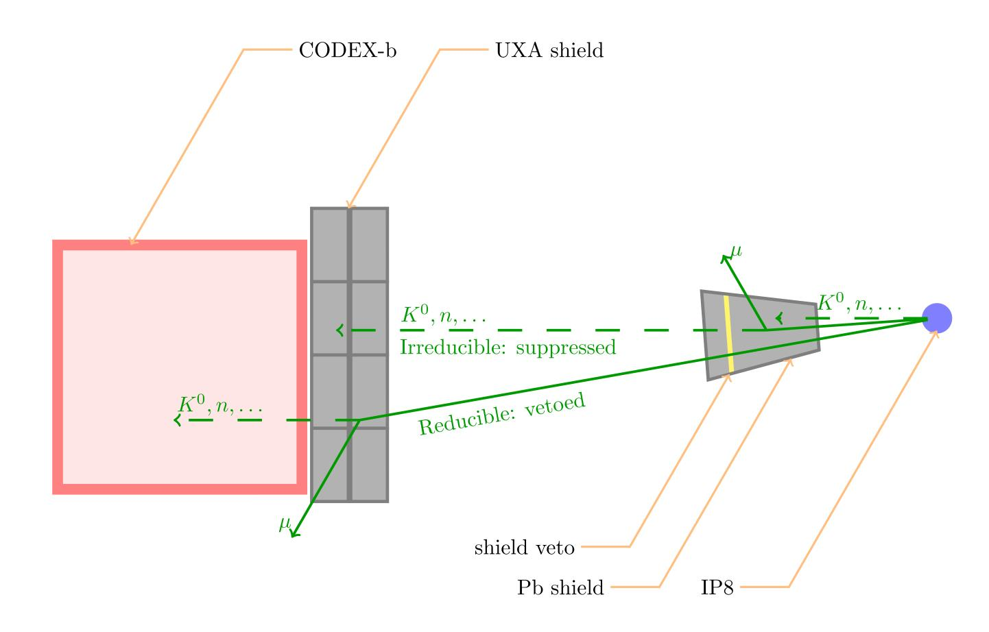
Simple design: use first part of the shield to attenuate muon & neutral hadron backgrounds which could enter the detector volume and scatter or decay within it, faking a signal. Then use a thin veto layer to eliminate secondary production of backgrounds within the shield itself.
