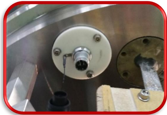
Fischer connectors: 4 fibers each connector
