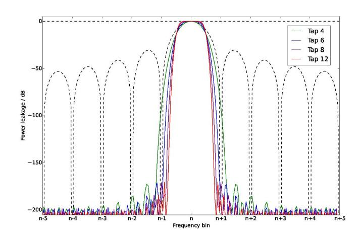
The dotted curve represents leakage due to a simple FFT.
