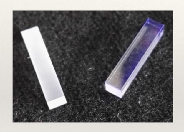
Optical treatment of the lateral surfaces of the crystals: **DEPOLISHING**.
