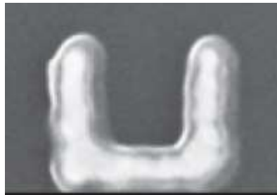
SRR structures: Photo of nanoscale split ring resonator structures fabricated in Bilkent University.
