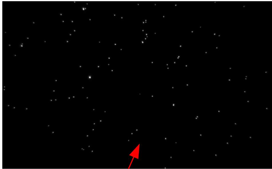
Image obtained with the protective cap mounted at the input of the image intensifier and at maximum amplification. The room was lit as usual.
