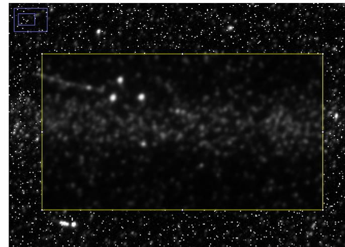
Image from  $5 \cdot 10^8$ , 300 MeV/u  $^{238}\text{U}^{73+}$  ions in  $\text{N}_2$ ,  $p = 5 \cdot 10^{-3}$  mbar.
