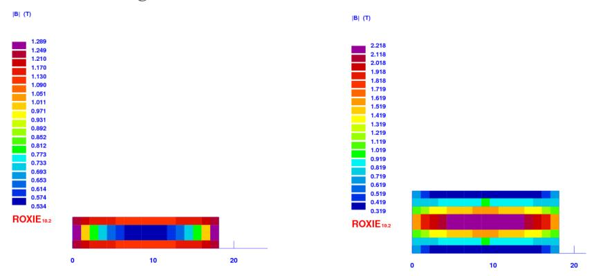
Peak field in the busbars, one busbar (left) and two positive/negative busbars (right)
