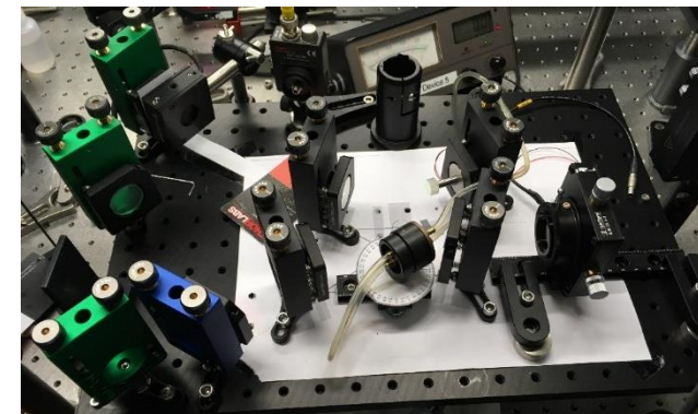
New TiSa bow-tie (ring) cavity for high resolution
