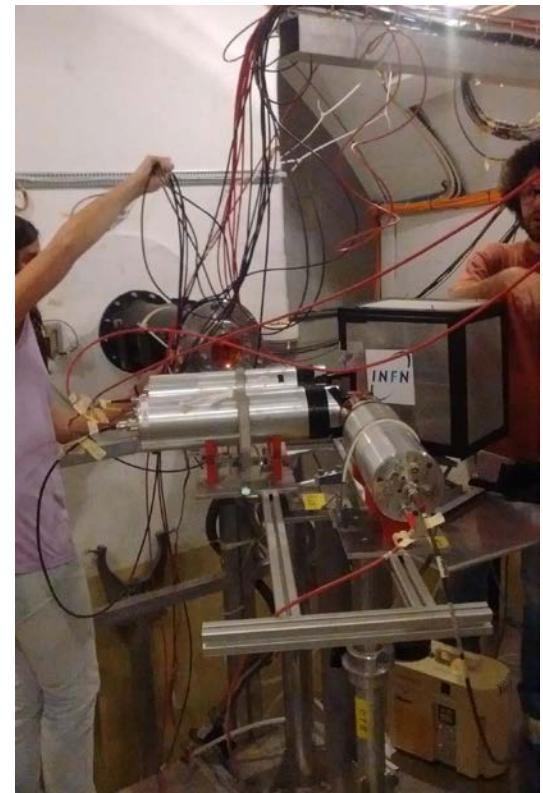
NB: Alignment of RPTs to the neutron beam was not perfect
