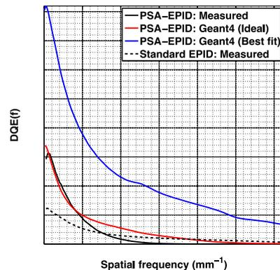
Figure 2. DQE measured with the prototype PSA-EPID and simulated using the Geant4 model. Simulation results were generated using ideal values for the uncertain parameters as well as values that best fit the measured data. The DQE measured using a standard commercial EPID is also shown for comparison.
