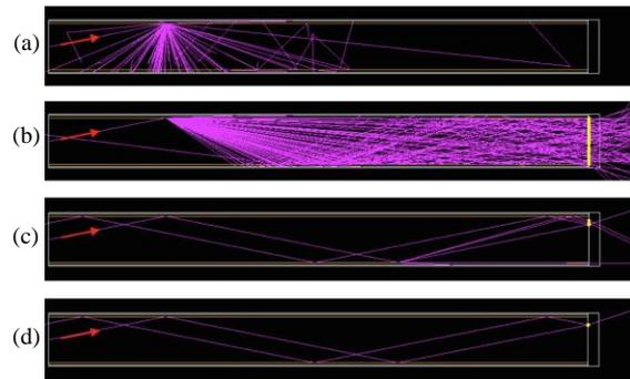
Figure 1. Visualisations showing 100 optical photons (incident from the red arrow) propagating along a single fibre when simulating the core/cladding boundary as a: (a) polished reflector; (b) specular spike reflector; (c) specular lobe reflector; and (d) diffuse lobe reflector. Detected photons are indicated as yellow dots.
