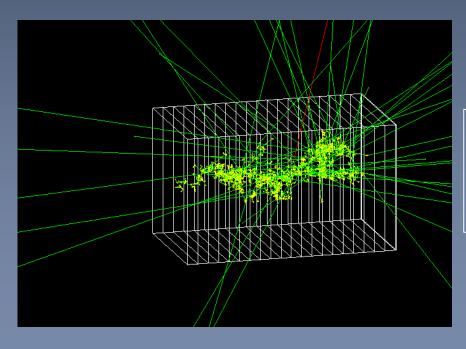
Incident neutron in concrete block with biasing activated. Slices on this figure are in the parallel geometry
