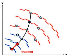
Form a tracklet with two stubs from neighbouring layers and propagate the tracklet to construct the track
