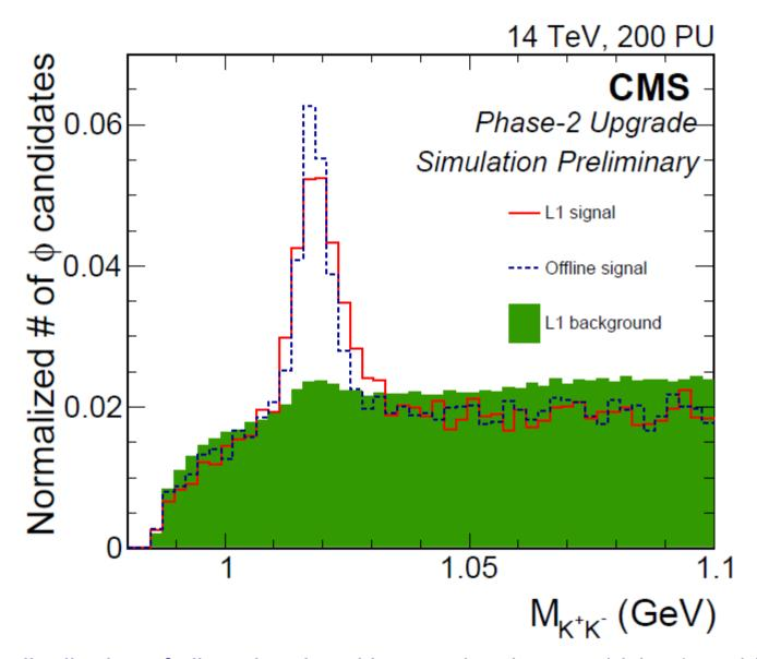
Invariant mass distribution of all track pairs with opposite charges,  $|d_z| < 1 \text{cm}$ ,  $|d_{xy}| < 1 \text{cm}$ , track  $p_T > 2 \text{ GeV}$ . Kaon mass assigned to all the tracks. The event sample does not have any preliminary selection on the  $B_s$  mass window. Distributions are normalized to unit area
