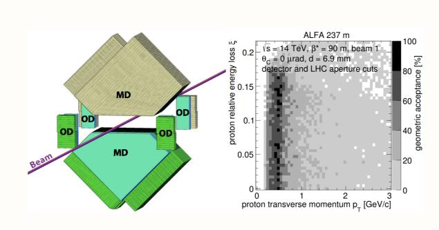
ular to the accelerator ring. They are equipped with planes of the scintillating fibres to measure the elastically scattered protons. Such measurements can be performed during the dedicated runs with high- $\beta^*$  optics.
