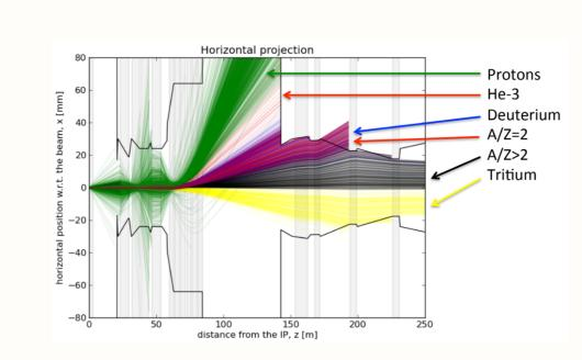
The are scattered into the accelerator beam pipe as nuclear fragments and can be detected by a dedicated set of detectors. Moreover, he use of the such detectors to veto nucleus disintegration is a very important experimental tool aiding selection of two-photon physics processes in HI interactions.
