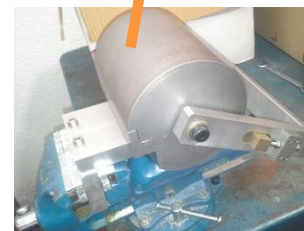
Collaring shoe preforming tooling
